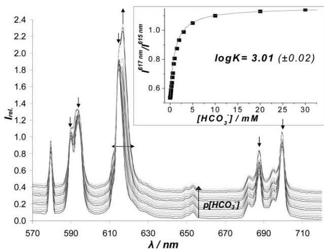
**Fig. 2** Variation of the Eu emission spectrum for  $[\text{Eu.L}^1]^{3+}$  following addition of sodium bicarbonate ( $\text{pH} = 7.4 (\pm 0.05)$ ;  $[\text{complex}] = 10 \mu\text{M}$ ;  $298 \text{ K}$ ,  $\lambda_{\text{exc}} = 384 \text{ nm}$ ;  $I = 0.1 \text{ M NaCl}$ ) showing (insert) a plot of the intensity ratio (617/615 nm) with  $[\text{HCO}_3^-]$ , allowing calculation of the apparent anion binding constant [ $\text{LV}_{\text{min}} 0.535$ ,  $\text{LV}_{\text{max}} 1.150$ ].
