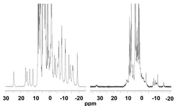
**Fig. 4**  $^1\text{H}$  NMR spectra for  $[\text{Eu.L}^{2a}]^{3+}$  in the absence (left) and presence (right) of 30 mM  $\text{NaHCO}_3$  (500 MHz, 295 K, pD 7.5, 1 mM complex).
