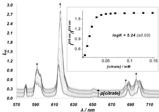
**Fig. 5** Variation of the europium emission spectrum for  $[\text{Eu.L}^{3a}]^{3+}$  in the presence of increasing concentrations of sodium citrate (pH 7.4, 0.1 M NaCl, 20  $\mu\text{M}$  complex, 298 K,  $\lambda_{\text{exc}}$  380 nm), showing (inset) the fit (line) to the observed data.
