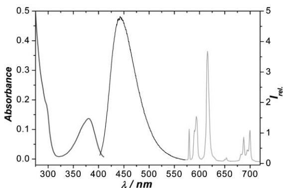
**Fig. 1** Absorption (left), chromophore fluorescence (centre) and Eu(III) emission (right) spectra for  $[\text{Eu.L}^1]^{3+}$  ( $\text{H}_2\text{O}$ , pH 7.4,  $10 \mu\text{M}$  complex).
